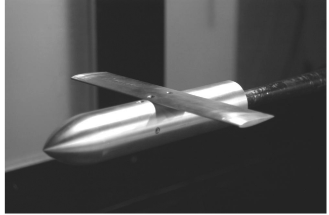
Fig. 3 Wing-body model in wind tunnel, AR = 5 , d/b = 0.2 .
